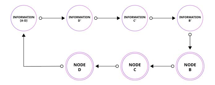
Unless Node B and Node C are controlled at the same time, it is almost impossible to know that Node A is sending a message to Node D.
